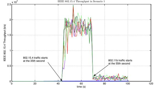
Fig. 5. Throughput of IEEE 802.15.4 nodes before and after IEEE 802.11b interference occurs in Scenario 1
