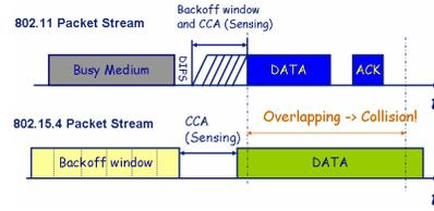
Fig. 3. In scenario 2: IEEE 802.11b/g nodes fails to sense IEEE 802.15.4 nodes
